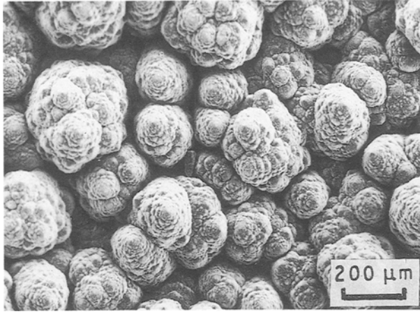
Figure 8 SEM surface morphology of CVD \beta -SiC dome-shaped structure with screw dislocations.
